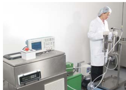
Pulsed Electric Fields Processor at Food Science Australia
