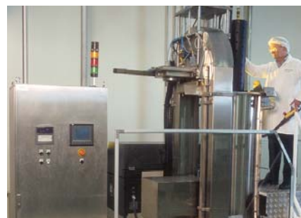
35 Litre High Pressure Processing unit at Food Science Australia
